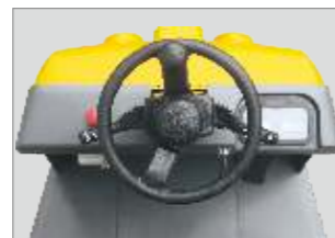
Adjustable steering column with electric F/R lever.
