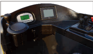
Camera and positioning: Optional positioning system offers easier pallet handling at height through camera system.
