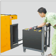
Rapid and simple battery changing system (option)
