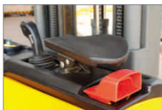
Finger-tip joystick and adjustable arm support
