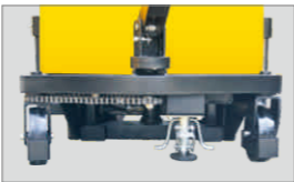
Chain Assist Steering System
