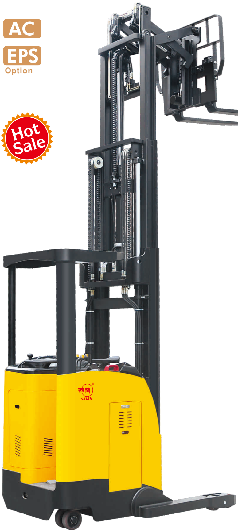
Vertically mounted drive motor with CANbus technology reduces wiring complexity and increase reliability.
