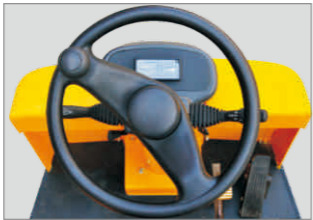
Adjustable steering column with electric F/R lever.
