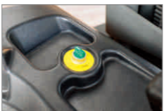
Manual or automatic stabilizers switch
