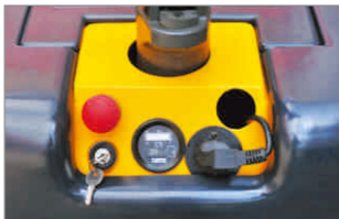
Multi-function Display, Built-in Charger
