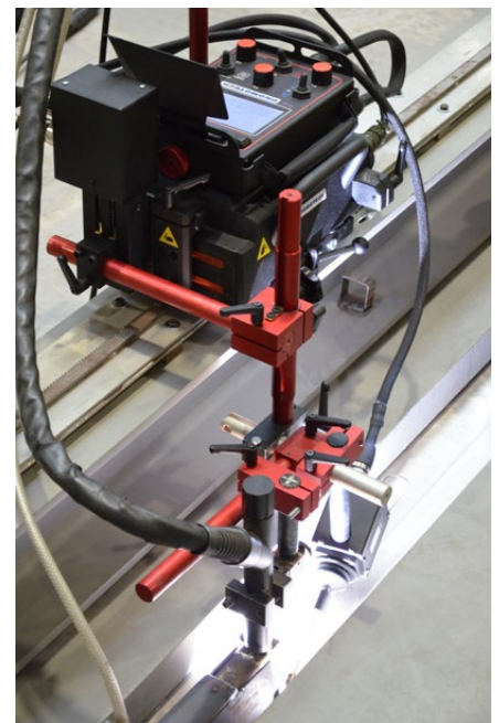
Seam tracking works with and without oscillation
