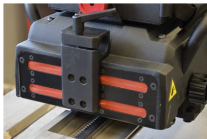
Silicone covers protect against dirt and spatter
