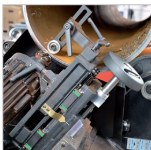
WSP-0436-24-00-00-0 Oval pipe tracking attachment (enables consistent land/root face thickness) Available either with brand new machine or for retrofitting
