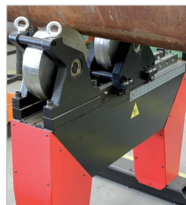
Heavy-duty adjustable pipe support ( \varnothing 200–1000 mm)
