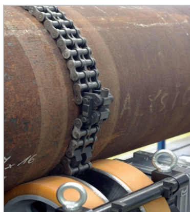
Adjustable chain ( \varnothing 200–1000 mm) ensures positive axial rotation
