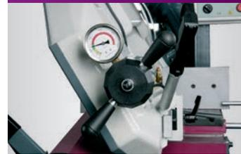
› Easy and accurate adjustment of the saw band tension by pressure gauge
