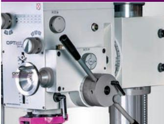
› Drilling depth stop adjustable within range of 0-120 mm. The feed is automatically switched off after reaching the preset drilling depth and turned back to its original position by the spring force of the return spring
