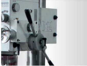
› Drilling depth stop adjustable within range of 0-120 mm. The feed is automatically switched off after reaching the preset drilling depth and turned back to its original position by the spring force of the return spring
