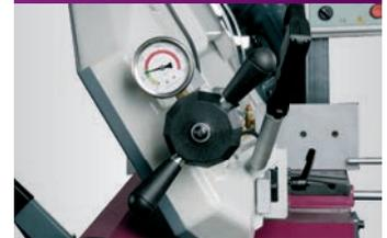
› Easy and accurate adjustment of the saw band tension by pressure gauge
