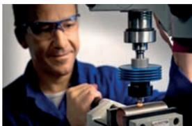
In thermal drilling, the friction heat from the existing material is used to create an anti-twist protected bushing without material removal in which a thread is then tapped.
