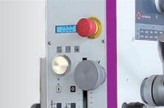
› Depth selection optionally in mm or inch and zero point freely adjustable via the display
