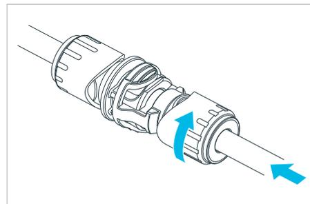
Push the pipe into connector, up to pipe stop. Twist locking cover 1/4 turn clockwise to prevent accidental pipe release (cover aligns with profile on body).
