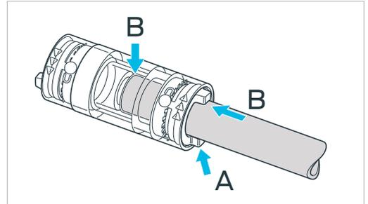
A – Connectors are supplied in the locked position, ready to use.
