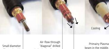
Electrode with "screw" holes in the direction of the "screw"
