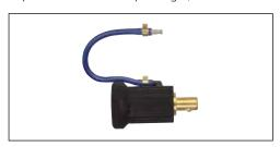
For torches with separate gas to be connected to power sources with central gas, use **W000306141**.
