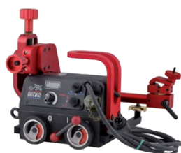
GECKO • Continuous welding • Dual torch welding
