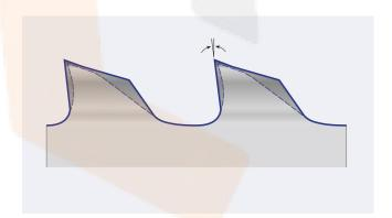
try. The innovative new production procedure with Superfinishing significantly extends the carrier band's lifetime, thus reducing the risk of bandbreakage. The optimized tooth cutting sharpness as well as a special limitation lead to an increased efficiency.
