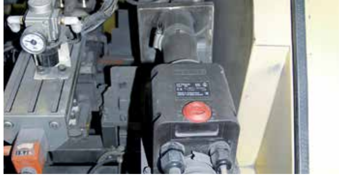
Deflashing foil sleeves from charcoal filter elements
