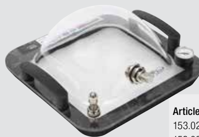
For testing T-joints
