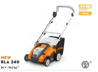
Compact cordless aerator for scarifying and combing smaller areas of lawn. Central adjustment of the working depth using a rotary switch on the housing, handlebar with 4-setting height adjustment, 34 cm working width, 16 blades. Includes scarifying blade, spring tine roller and 50-litre grass catcher box. Working area covered with recommended AK 30 battery is 250 m².
