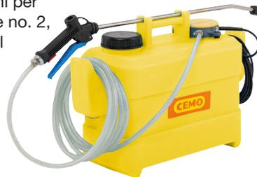
Spray lance with flat fan nozzle no. 4, spraying angle 110°, approx. 1040 - 1370 ml per minute flow rate, and flat fan nozzle no. 2, spraying angle 110° approx. 800 - 1000 ml per minute flow rate
