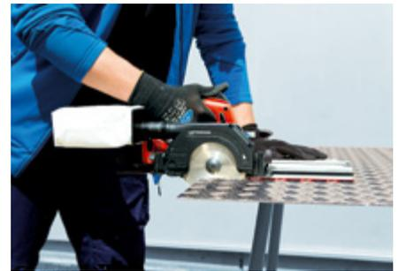
Cross cut guide rail (No. 1500003694) for cutting plates optionally available
