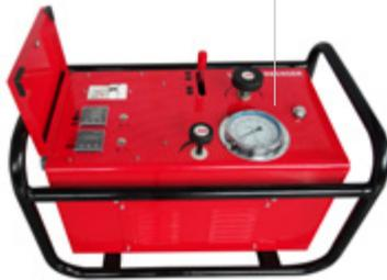
Supply of power for heating element and trimmer unit by the hydraulic. Additional plugs for external data logger (optional accessories)
