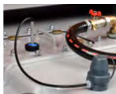
Including electronic overflow prevention sensor
