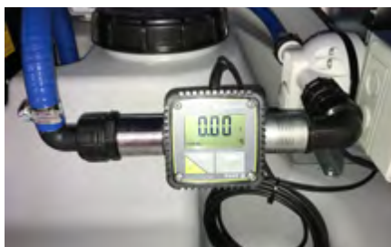
Meter FMT 3 with pulse output
