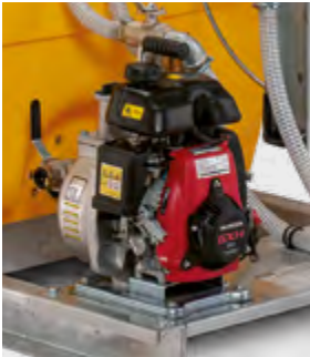
Honda pump with petrol engine 130 L/min
