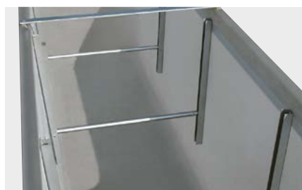
Large container: Hot dip galvanised external braces for above ground installation. Stainless steel internal braces for installation in the ground.
