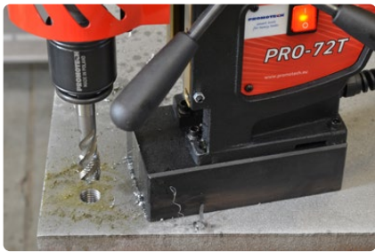
Tapping through holes up to M20
