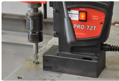
Tapping blind holes up to M20
