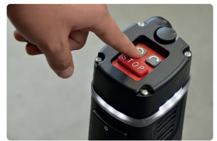
Counterclockwise (CCW) rotation User-friendly control of tapping tool retract
