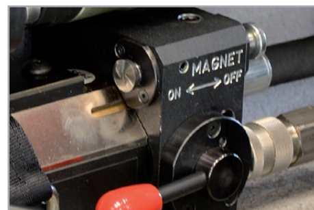
Protection against motor start-up when magnetic base is not activated
