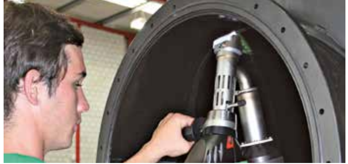
Even inside radiuses are easy to weld.
