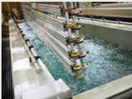
Galvanic bath made of polypropylene © Collini www.collini.eu
