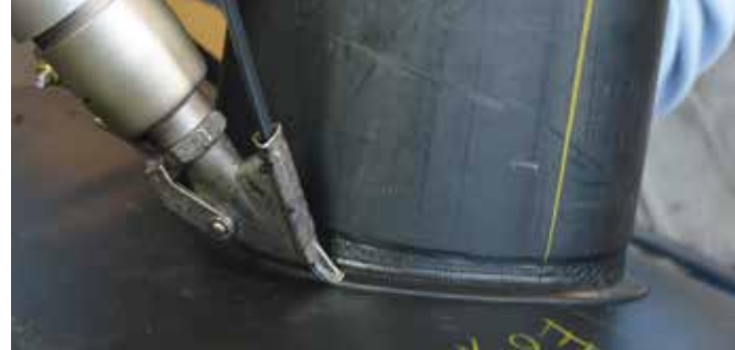
Draw welding with combination nozzle.
