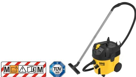
**REMS Pull M Set**, dry and wet extractor, certified as extractor and dust extractor for extracting health hazardous dusts in accordance with EN 60335-2-69 Dust class M. Exposure limit/work place limit > 0.1 mg/m³, penetration level ≤ 0.1 %.
