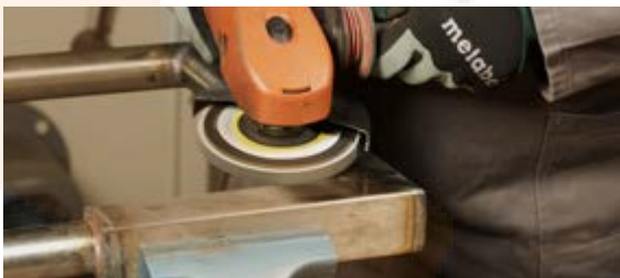
Removal of tempering colours and pre-polishing
