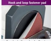
Good grinding wheel adhesion, easy replacement
