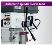
> Drilling depth stop adjustable within range of 0-85 or 105 mm. The feed is automatically switched off after reaching the preset drilling depth and turned back to its original position by the spring force of the return spring
