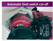
Switches the saw band off at the bottom stop
