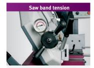
> Easy and accurate adjustment of the saw band tension by pressure gauge
