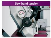
> Easy and accurate adjustment of the saw band tension by pressure gauge
