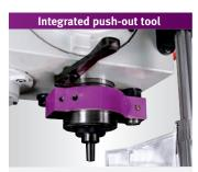
Spindle lock with integrated ejector for easy tool change
