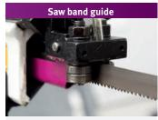
Ball-bearing borne; for an excellent band run and thus optimal cutting
