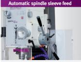
> The spindle sleeve moves downwards at the set feed speed and switches off again at the set drilling depth on the scale ring. The spindle sleeve then moves back to its starting position.
