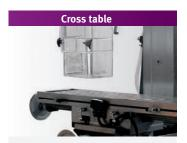
The cross table (X-axis) can be rotated through ± 45°
