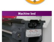
> Grey cast iron prism bed with strong ribbing, aged for at least six months, induction tempered and precision ground
