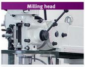
> The spindle head can be swivelled forwards or backwards through 45° and swivelled through 90° to the right or left
