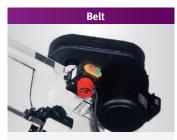
Four speeds adjustable by shifting the belt
