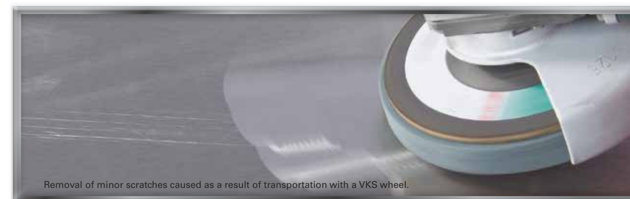
Deep scratches are fully removed. Only very slight traces of disc rotation may remain. If required subsequent steps can be carried out using a burnishing machine with various grades of nylon web grinding wheels (speed setting 1-2*) or pyramid sanding belts (speed setting 5*) to achieve a perfect linear finish.
