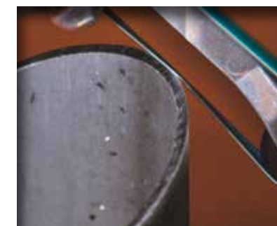
Effective deburring the coarse nylon web fleece belt on speed setting 6*.
