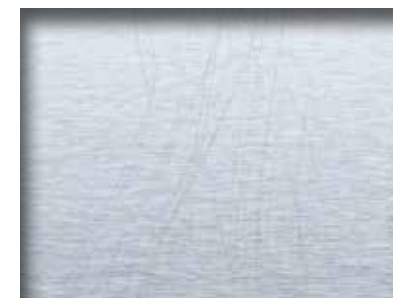
Minor scratches to the surface caused by transportation
