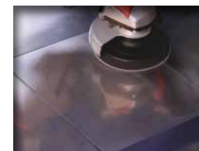
Remove scratches with a soft backing pad, e.g. (M14 6.23300) fitted with a Pyramid cling-fit sanding sheet, e.g. 6.26374 (speed setting 3*). The soft disc will help prevent any undulations forming in the surface material.
