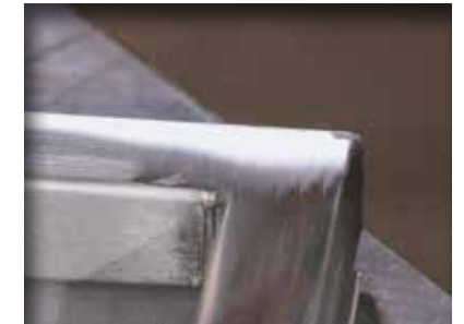
Weld seam removed. Turn to the next page for further steps.
