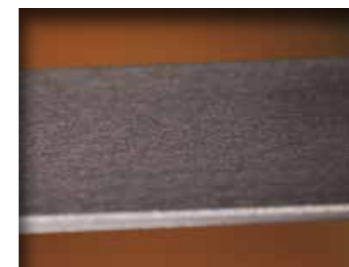
Coarse longitudinal finish left after the surface skin has been 'opened'.
