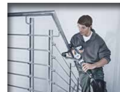
With a nylon web fleece belt select half speed setting 3* and get a transition-free satinised result.
