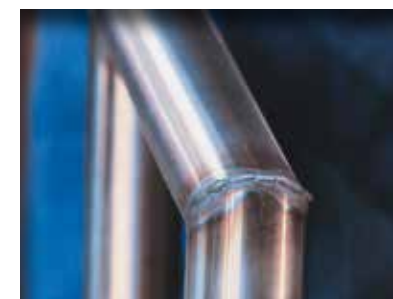
TIG welding seam on a handrail corner.
