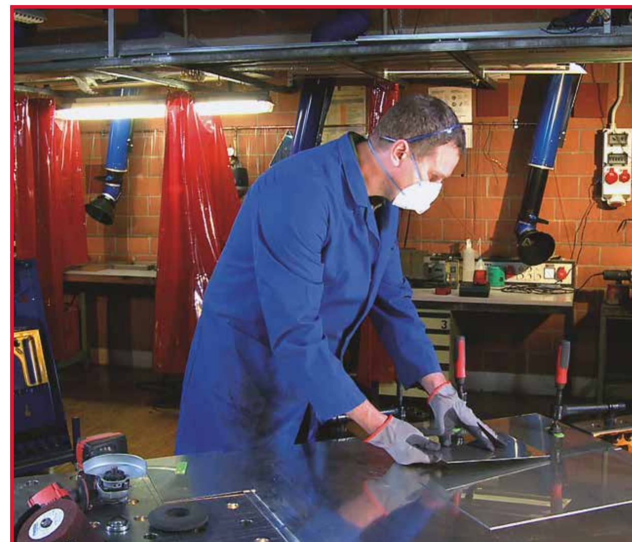
Using the SE 12-115 with the P 180 6.23499 rubber sanding roller on speed setting 1*.
