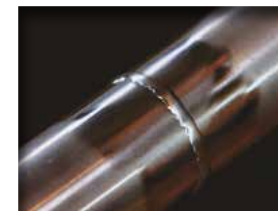
Slightly rounded welding seam, the tarnish has been removed.
