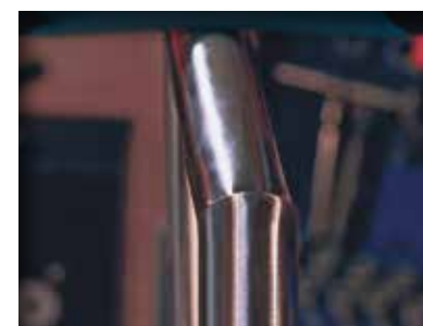
Traces of rotation marks from the weld removal stage of the process, e.g. from the steps seen on page B 5. Grinding welding seams.
