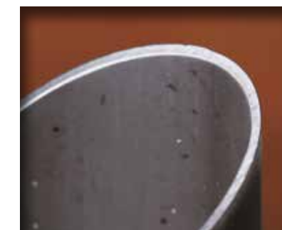
A pipe that has been deburred fully both inside and out.
