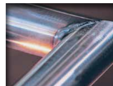
Right angle weld seam on a handrail.
