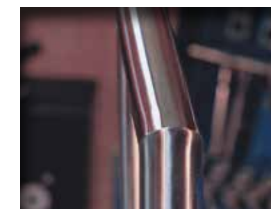
Matched satin finish, rotation traces from the pre-grinding process have been eliminated.
