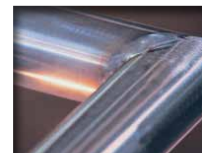
Ground fillet weld seam with perfect transitions.
