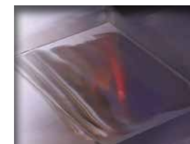
Deep scratches are fully removed. Only very slight traces of disc rotation may remain. If required subsequent steps can be carried out using a burnishing machine with various grades of nylon web grinding wheels (speed setting 1-2*) or pyramid sanding belts (speed setting 5*) to achieve a perfect linear finish.
