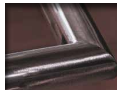
Minor structural grooves on the handrail corner can be seen.
