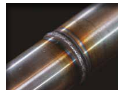
Typical tarnish related to a TIG welding seam
