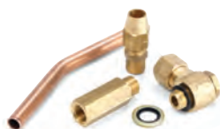
11 Supplementary cooler, to be used where the inlet water temperature is higher than 25°C or the outlet water flow from the machine is lower than 5 l/min
