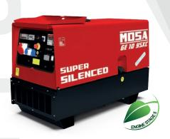
**ENGINE - 4-STROKE, INDIRECT INJECTION, NATURAL ASPIRATED** YANMAR 3TNV80F Fuel consumption (75% of PRP) 1.8 lt./h **Tank capacity** 30 I Alternator synchronous three-phase, self-excited, selfregulated, brushless Stand-by Three-phase power 9.5 kVA (7.6 kW) / 400V / 13.7 A PRP Three-phase power 9 kVA (7.2 kW) / 400V / 13 A PRP single-phase power 4.5 kVA / 230V / 19.5A **Dimensions Lxlxh (mm)** 1460x700x920 mm Dry weight 410 kg **Acoustic pressure** 62 dB(A) @ 7m
