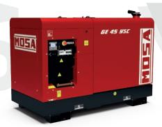
YANMAR 4TNV98T Fuel consumption (75% of PRP) 7.4 lt./h Tank capacity 55 L Alternator synchronous three-phase, self-excited, selfregulated, brushless Stand-by Three-phase power (LTP) 44 kVA (35.2 kW) / 400 V / 63.5 A PRP Three-phase power 40 kVA (32 kW) / 400 V / 57.7 A PRP single-phase power 15.5 kVA / 230 V / 67.4 A Dimensions Lxlxh (mm) 1800x900x1333 mm Dry weight 880 kg **Acoustic pressure** 70 dB(A) @ 7m
