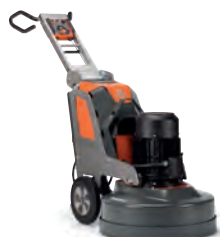
ELECTRIC-POWERED HUSQVARNA PG 830 S 11 kW, 380-415 V, 3-phase, grinding width 800 mm, grinding disc 3×270 mm, 497 kg.
