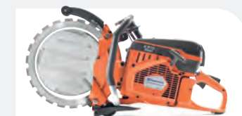
PETROL-POWERED HUSQVARNA K970 RING 94 cc, 4.8 kW, 13.8 kg, blade size 370 mm, cutting depth 270 mm.
