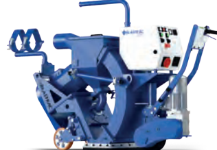
ELECTRIC-POWERED HUSQVARNA BLASTRAC 1-15DS 15 kW, 400 V, 63 A, working speed 0.5–25 m/min, working width 380 mm, 450 kg.
