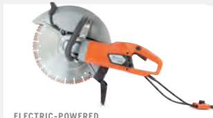
ELECTRIC-POWERED HUSQVARNA K4000 230/120/110 V, 2700/1800/2200 W, 8.5 kg (incl. Vac attachment 1 kg), blade size 350 mm, max. cutting depth 125 mm.
