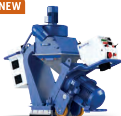
ELECTRIC-POWERED HUSQVARNA BLASTRAC EBE 500E 22 kW, 400 V, 63 A, working speed 1–15 m/min, working width 500 mm, 742 kg.
