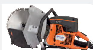
PETROL-POWERED HUSQVARNA K770 VAC 74 cc, 3.7 kW, 11.0 kg, blade size 300 mm, cutting depth 122 mm.
