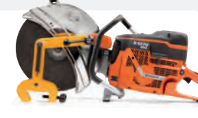
PETROL-POWERED HUSQVARNA K1270 RAIL 119 cc, 5.8 kW, 20.5/21.2 kg (incl. RA10), blade size 350/400 mm, cutting depth 118/145 mm.
