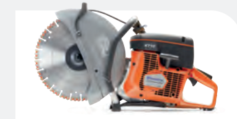
PETROL-POWERED HUSQVARNA K770 / K770 WITH OILGUARD 74 cc, 3.7 kW, 10/10.1 kg, blade size 300/350 mm, cutting depth 100/125 mm.
