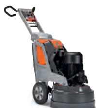
ELECTRIC-POWERED HUSQVARNA PG 690 12.5 kW, 380-415 V, 3-phase, grinding width 640 mm, grinding disc 3×270 mm, 502 kg.
