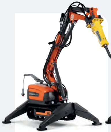
HYDRAULIC-POWERED HUSQVARNA DXR 315 27 kW, 2020 kg, reach 5.5/5.2 m up/forward incl. tool.
