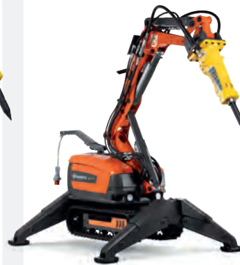
HYDRAULIC-POWERED HUSQVARNA DXR 275 24 kW, 1750 kg, reach 4.8/4.5 m up/forward incl. tool.
