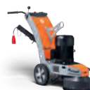
ELECTRIC-POWERED HUSQVARNA BG 250 5.5 kW, 400 V, 3-phase, grinding width 250 mm, 146 kg.
