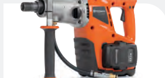
DRILL MOTOR HUSQVARNA DM 540i 1350 W, recommended drill diameter 15–75 mm (100 mm with drill stand), 4.9 kg.
