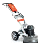
ELECTRIC-POWERED HUSQVARNA PG 450 1.5/2.2 kW, 110/230 V, 1-phase, grinding width 450 mm, grinding disc 3×180 mm, 109 kg.
