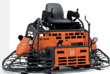
PETROL-POWERED HUSQVARNA CRT 48 PS Ideal for finishing surfaces 1000–2300 m 2 . The power steering enables accurate manoeuvring and virtually fatigue-free operation with two control modes to accommodate operator preference in varying site conditions. 42.5 kW, 2×1220 mm, 660 kg.
