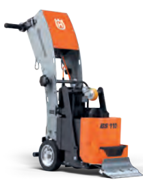
ELECTRIC-POWERED HUSQVARNA BS 110 0.75/1.5 kW, 110/230V/16 A, 170 kg.
