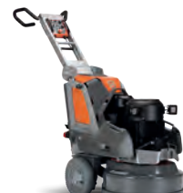
ELECTRIC-POWERED HUSQVARNA PG 690 RC 12.5 kW, 380-415 V, 3-phase, grinding width 640 mm, grinding disc 3×270 mm, 598 kg.
