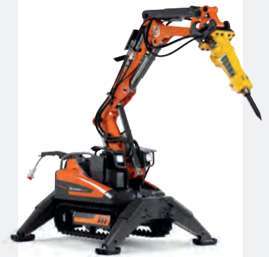
PETROL-POWERED HUSQVARNA DXR 145 18.5 kW, 985 kg, reach 4.4/3.7 m up/forward incl. tool.
