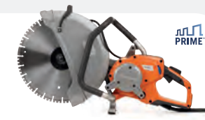
ELECTRIC-POWERED HUSQVARNA K7000 400 V, 5.5 kW (3-phase), 9.8 kg, blade size 400 mm, cutting depth 155 mm.
