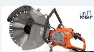
ELECTRIC-POWERED HUSQVARNA K7000 SMARTGUARD 400 V, 5.5 kW (3-phase), 10.8 kg, blade size 400 mm, cutting depth 155 mm.
