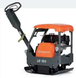
DIESEL-/PETROL-POWERED HUSQVARNA LG 164 3.1–3.6 kW, 148–170 kg.
