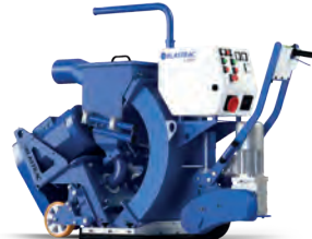
ELECTRIC-POWERED HUSQVARNA BLASTRAC 2-20DT 2×11 kW, 400 V, 63 A, working speed 0.5–33 m/min, working width 550 mm, 575 kg.
