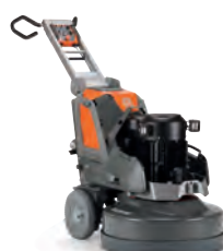
ELECTRIC-POWERED HUSQVARNA PG 830 RC 16.5 kW, 380-415 V, 3-phase, grinding width 800 mm, grinding disc 3×270 mm, 652 kg.
