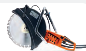
HYDRAULIC-POWERED HUSQVARNA K2500 150 bar/40 l/min, 5.2 kW, 8.3 kg, blade size 400 mm, cutting depth 145 mm.
