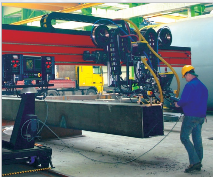
Standard Column & Boom with ESAB Aristo 1000 AC/DC
