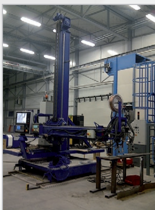
Standard Column & Boom with ESAB Aristo 1000 AC/DC
