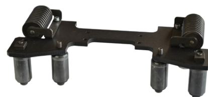
Round plate beveling attachment: Minimal outer radius R=1000 mm (40") Minimal inner radius R=1000 mm (40") Max bevel width 19 mm Product code: ZSP-0539-10-00-00-0
