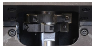
2 rotary milling heads, each holding five 4-sided indexable inserts
