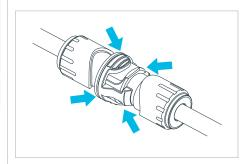
Firmly push the opposing ends of connector together, until latched, activating internal gas blocking mechanism.
