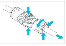
To release the pipe twist the locking cover 1/4 turn anti-clockwise, push the collet square against the face of the connector, then remove the pipe (cover misaligns with profile on body). Depress yellow catch to release gas block.
