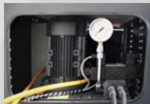
Dual-circuit hydraulic unit in cabinet base
