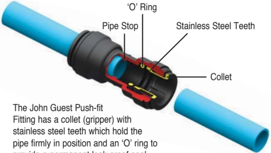
The John Guest Push-fit Fitting has a collet (gripper) with stainless steel teeth which hold the pipe firmly in position and an 'O' ring to provide a permanent leak proof seal.
