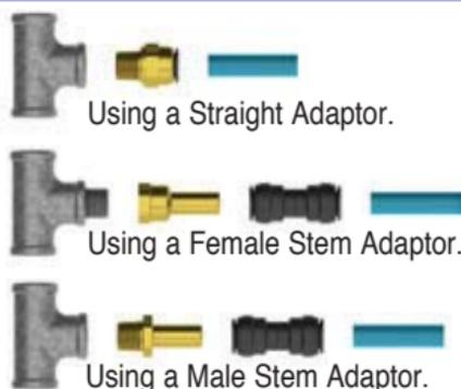
John Guest fittings and pipe can form a stand alone system or be used to modify or extend an existing galvanised system.
