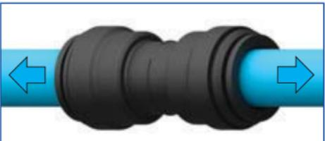
**To disconnect,** ensure the system is depressurised. Push the collet towards the fitting and remove the pipe. The fitting can be reused.
