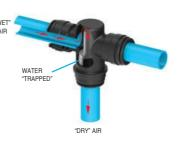
The ingenious inside arrangement of the fitting allows air to flow, with minimum head loss, from the main to take-off point without allowing water to follow. The moisture is retained in the line to be drawn off at some suitable location.
