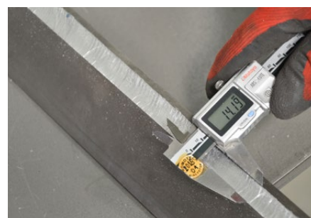
Maximum bevel width up to 14 mm
