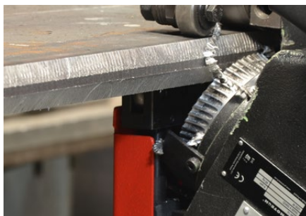
Bottom plate beveling
