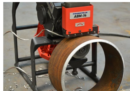
Oval workpiece and pipe beveling
