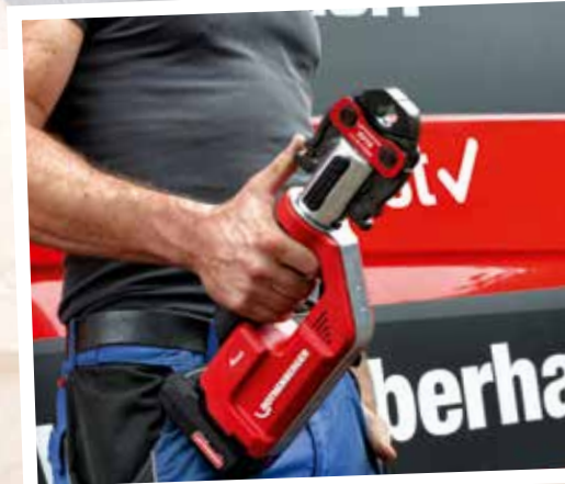
Secondary effect of the two-cylinder-structure: The machine can be used with one hand.
