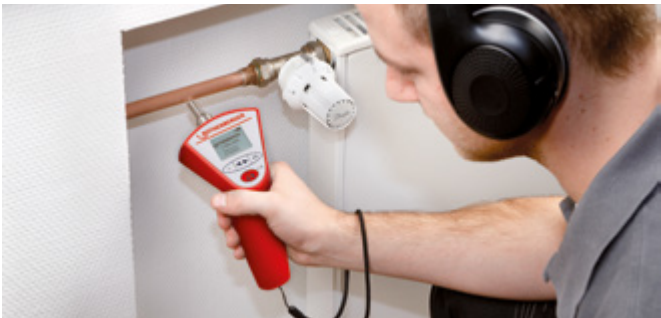
Acoustic leak detection of heating installations
