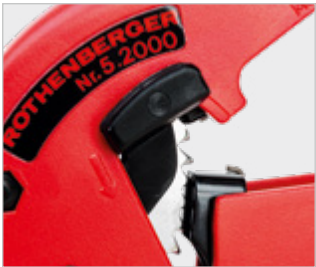
Ideally meshed cutting curve
