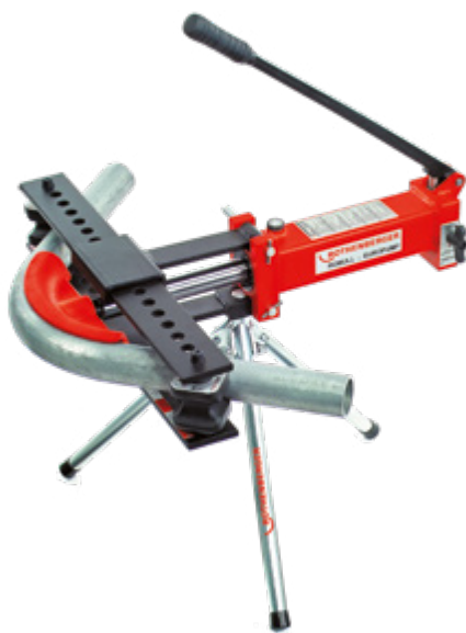
ROBULL type E with foldable bending frame
